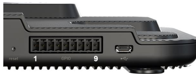
Figure 8: Impinj R700 Series GPIO Pin Locations
